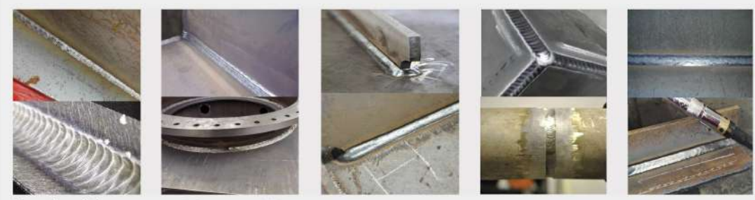
Bevel multipass welding Multipass welding Corner welding Solid wire welding Flux-cored arc welding
